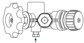
1/8" F.NPT Pressure Test Port is isolated from the container when the service valve is closed.
